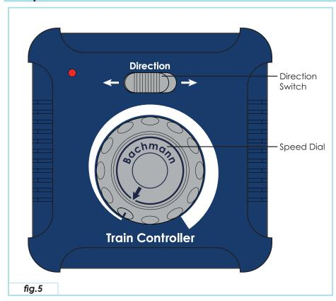
The Bachmann Train Controller features a Speed Dial and a Direction Switch. (fig.5)
