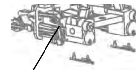
The valve guides fit into the holes in the back of the cylinder chest as indicated. There are two spare items included in the packet. Draincocks fit under the cylinders
